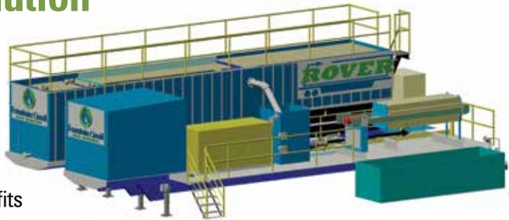
into all on-site completion and water management equipment within a single day. Once installed, produced water is pumped into the ROVER™ from a source — frac tank, SWD or pit. We use an adjustable chemical system and a proprietary polymer blend to flocculate suspended solids and organics. The solids settle on the bottom of our built-in sludge thickener, where they are continuously collected and removed. Clean brine is pumped out of the unit to our customer's designated storage location.
